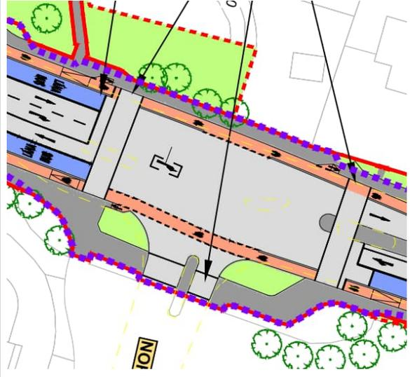
Junction Type 1, which accommodates an inbound and an outbound bus lane, is proposed on the CBC mainline. Both bus lanes extend to the stop line, which provides greater bus priority and reliability..
